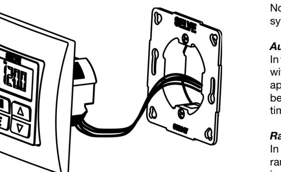
Fix the holding frame in the flush-mounted socket. Finally insert the device into the holding frame
