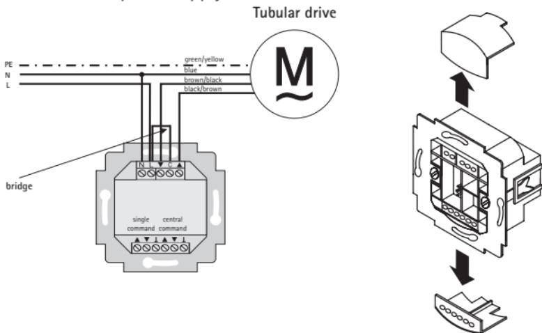
2. Put the protective caps back on the power supply unit.
