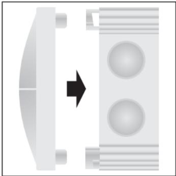
5) Replace the cover and turn the screws into position 1.
