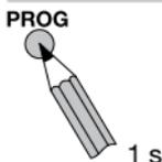
To save the programmed transmitter, press the **PROG** key for one second. The transmitter is now permanently programmed in the receiver.
