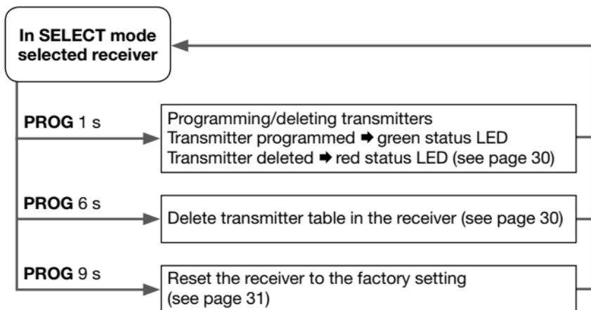
**Note for settings under point 6.2.:** The receiver must be selected for this setting with a transmitter in **SELECT** mode (Status LED flashes slowly in orange). After completing the setting, the motor/receiver is still selected (see point 6.).
