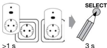
1. Interrupt the voltage supply of the receivers for > 1 second. The receivers can be found within the next 4 minutes.
